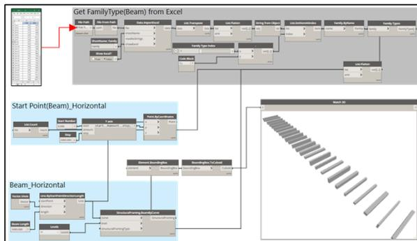
Figure 3. Parametric modeling using Revit Dynamo
